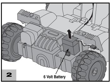
Lift to remove the battery from the battery compartment.
