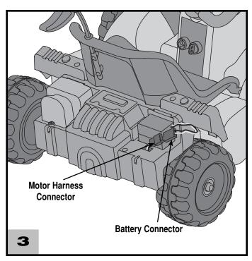
• Plug the battery connector into the motor harness connector. **Note:** If the battery connector will not plug into the motor harness connector, turn it over and try again. Do not force the battery connector into the motor harness connector.
