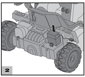
Place a Power Wheels<sup>®</sup> 6 volt (4.0 Amp/Hr.) battery upright in the battery compartment, as shown.
