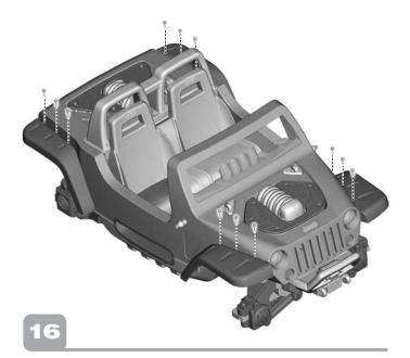
• Fit three screws into the top of each fender and tighten.
