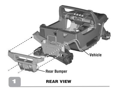
• Fit the rear bumper to the rear end of the vehicle.
