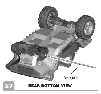
• Slide the rear axle through the large opening near the rear of the vehicle, as shown.
