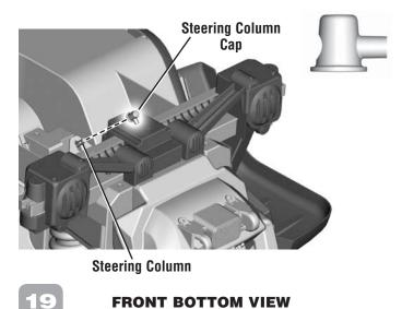
• Fit the steering column cap onto the end of the steering column.
