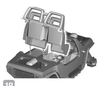
• Insert the tabs on the front edge of the seat into the slots inside the vehicle.
