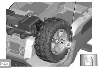
• Fit a wheel retainer onto the end of the rear axle.
