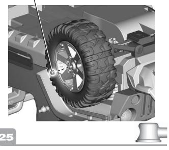
• Fit a front axle cap onto the end of the front axle.
