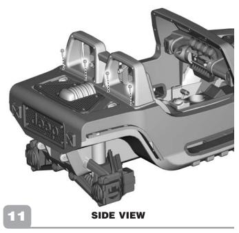
• Insert four screws through the seat bar and into the vehicle. Tighten the screws.
