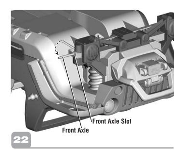
• Turn both front axles torward the front end of the vehicle until they drop into the axle slots.
