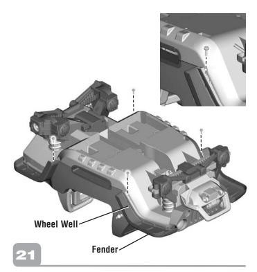
• Insert a screw through each wheel well and into each fender. Tighten the screws.
