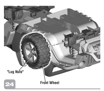
**Note:** There are front and rear wheels. The rear wheels have a grooved hub while the front wheels do not.
