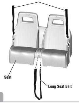
• Insert the fastener end of a short seat belt strap through the slot near the outer edge of the seat. Make sure the side of the seat belt with the fastener faces the outer edge of the seat.
