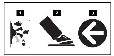
**IMPORTANT!** To avoid damaging the motors and gears, stop the vehicle before shifting from forward to reverse.
