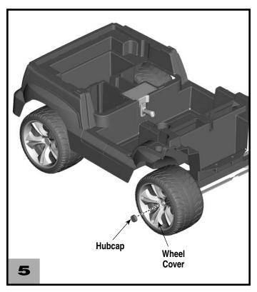
• Align the slot in a hubcap with the rib in the wheel cover. "Snap" a hubcap into the center of each wheel cover.
