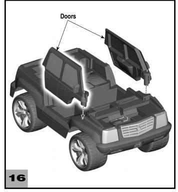
• Fit the door pegs onto the holes near the front end of the vehicle. *Hint:* There is a left and right door. They are designed to be assembled one way.
