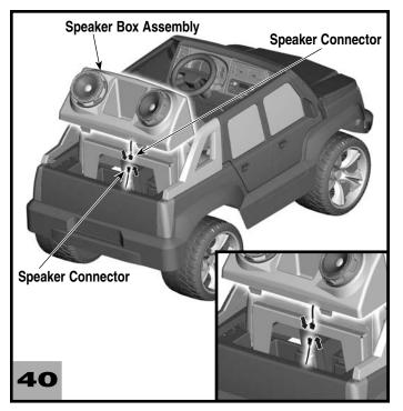
Position the speaker box assembly over the back end of the vehicle.Plug both speaker connectors together.
