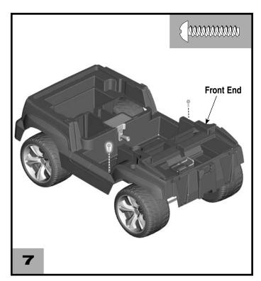
• Insert two #8 x 3/4" screws through the front end and into the vehicle. Tighten the screws.
