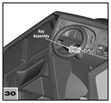
• Insert and "snap" the key assembly into the slot in the dash.
