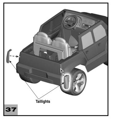
• Fit the taillights (left and right) onto the rear of the vehicle.
