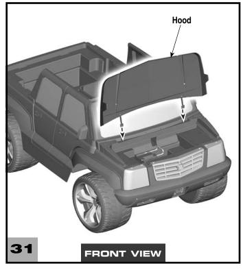
• Fit the long tabs on the hood into the slots in the front end of the vehicle.
