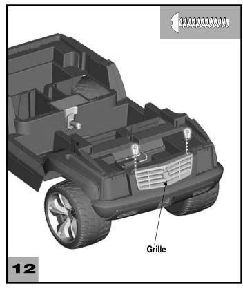
• Insert two  $\#8 \times 3/4"$  screws the top of the grille. Tighten the screws.
