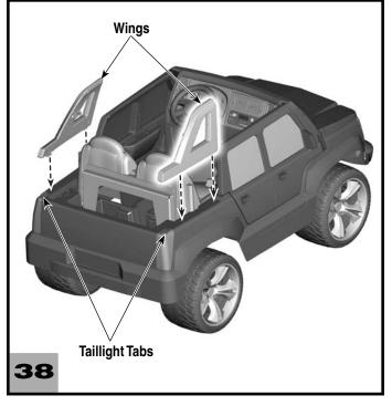
• Fit the wing tabs into the slots in the top edge near the rear of the vehicle.
