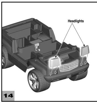
• Fit the headlights (left and right) onto the bumper.
