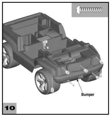
• Insert seven #8 x 3/4" screws into the bumper and tighten.
