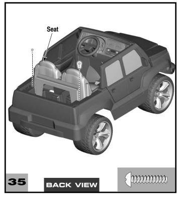
• Insert two #8 x 3/4" screws into the back of the seat. Tighten the screws.
