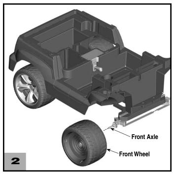
**Hint:** There is a right and a left front wheel. Place the right wheel (marked R) on the passenger side of the vehicle, and the left wheel (marked L) on the driver side of the vehicle.
