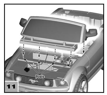
• Fit the dash assembly onto the posts near the front end of the vehicle.
