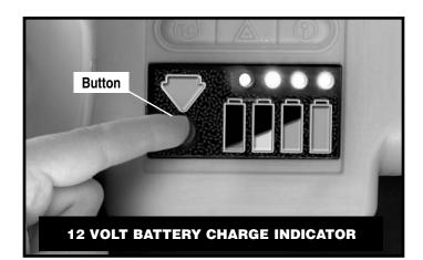
**IMPORTANT!** Do not press the 12 volt battery charge indicator while the vehicle is moving.
