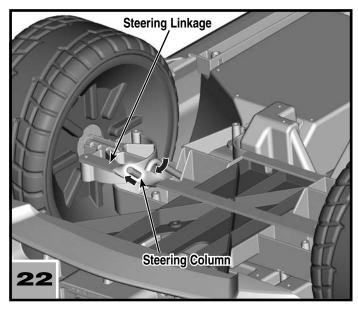
• Insert the curved end of the steering column though the hole in the steering linkage.
