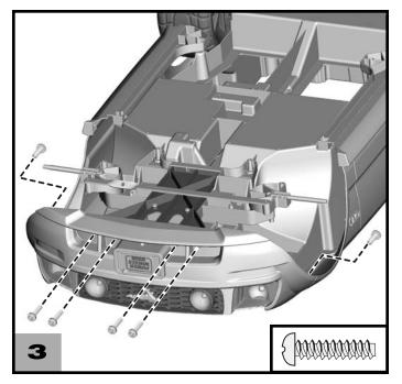
• Insert six #8 x <sup>3</sup>/<sub>4</sub>" screws into the front bumper and tighten.
