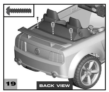
• Insert three black #8 x <sup>3</sup>/<sub>4</sub>" screws into the back of the seat and tighten.
