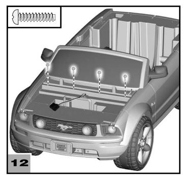
• Insert four #8 x <sup>3</sup>/<sub>4</sub>" screws into the dash assembly and tighten.
