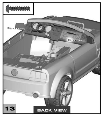
• Insert two black #8 x <sup>3</sup>/<sub>4</sub>" screws into the dash assembly as shown and tighten.
