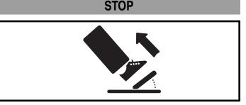
• Your vehicle has a patented, electronic braking system that automatically stops the vehicle when your child's foot lifts from the pedal. Make sure your child is comfortable with steering the vehicle and automatically knows how to stop.
