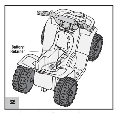
· Loosen the screw in the battery retainer and remove it.
