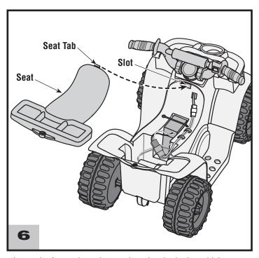
• Insert the front tab on the seat into the slot in the vehicle.
