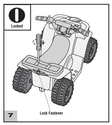
• Using a slotted screwdriver, turn the lock fastener 1/4 turn to the locked position ①.
