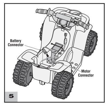
• Plug the battery connector into the motor connector. **Hint:** If the battery connector will not plug into the motor connector, turn it over and try again! Do not force the battery connector into the motor connector.
