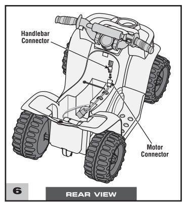
Plug the handlebar connector into the motor connector.
