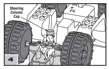
• "Snap" the steering column cap over the cap nut.
