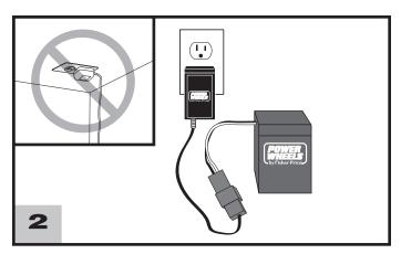
• Plug the charger into a standard wall outlet.
