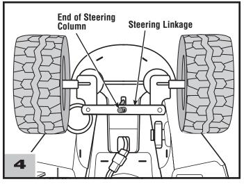
• Fit the end of the steering column through the hole in the steering linkage.
