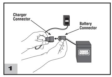
• Fit the charger connector and the battery connector together.
