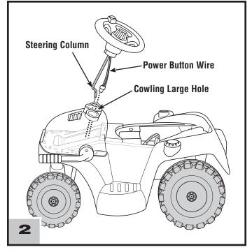
• Fit the steering column and power button wire into the large hole in the cowling. Make sure the steering column goes through the small slot inside the vehicle.
