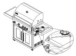
STEP 3: Battery is inserted for the rotisserie burner . To install the battery, turn the ignition button cap counterclockwise and remove it. Replace the ignition button cap after the battery is installed.
