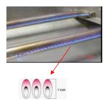
Visually check the burner flames prior to each use, the flames should look like this picture, if they do not, refer to the burner main tenancy part of this manual.
