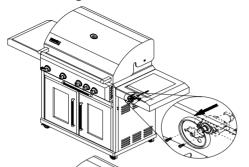
B. Push the side burner control knob into the valve steam and tighten it using the Allen Wrench.
