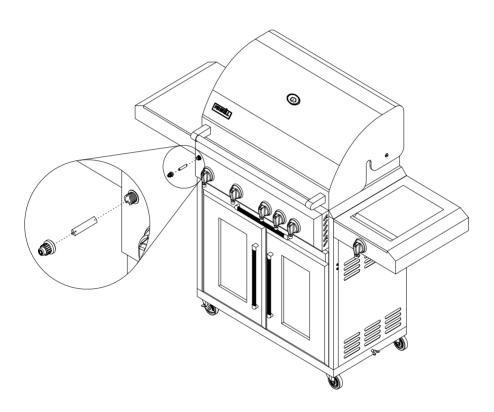
STEP 4: The screws for rotisserie drive motor bracket are attached to the motor bracket. Remove the screws and install the rotisserie motor bracket as shown in the figure below. Assemble the rotisserie skewer as shown in the figure below.
