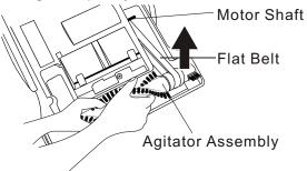
Place a new flat belt onto the motor shaft and pulley.
