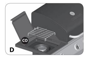
d. Place the side burner cooking grate (CO) into postion on the side burner shelf, as shown in figure E.
