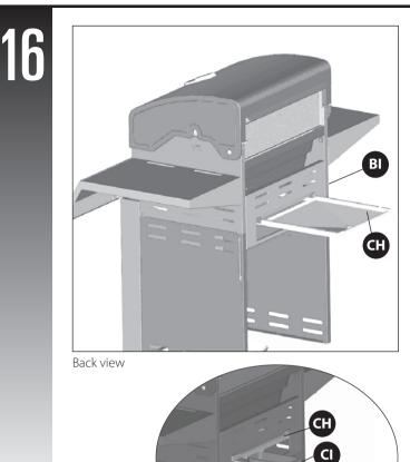
a. Insert the grease tray (CH) into the opening in the upper back panel (BI), making sure to engage tracks located under burner box.
