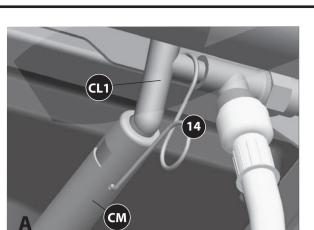
a. Use the side burner Venturi clip (#14) to connect the side burner (CM) to the side burner valve (CL1).
