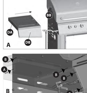
**TIP:** To position the left side shelf, insert the two hooks on the side shelf assembly into the two support brackets located on the upper left side panel (BB).
