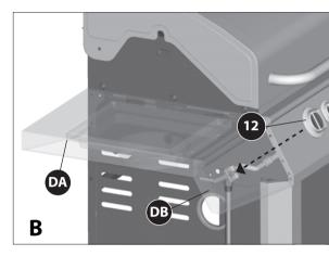
Remove the hardware that is pre-assembled to the side burner valve bracket (CC), as shown in figure A. Insert the side burner valve stem through the rear of the left side shelf fascia (DB). Assemble the side burner valve (CC) to the side shelf fascia (DB), using the hardware removed.
