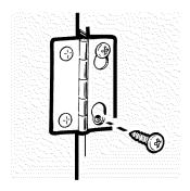
Remove the remaining screws from the side of the opening from which the door was removed. With these screws secure each hinge at the bottom. Tighten the two top screws of each hinge. Reinsert the plastic plugs on the side from which the door was removed.
