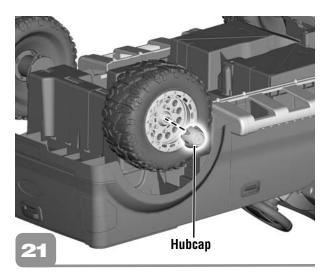
• Align the tabs on a hubcap with the slots in a rear wheel. "**Snap**" a hubcap into the center of the rear wheel.
