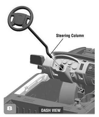
• Insert the end of the steering column down through the opening in the dash and down through the hole in the vehicle floor.
