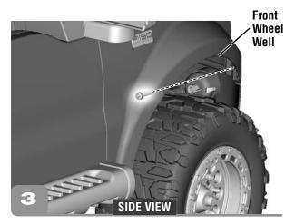
• Insert a screw through **both** front wheel wells and into the front grille. Tighten the screws.
