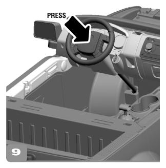
• Press the steering wheel down to "snap" into place.
