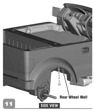
• Insert a screw up through both rear wheel wells and into the cargo bed. Tighten the screws.
