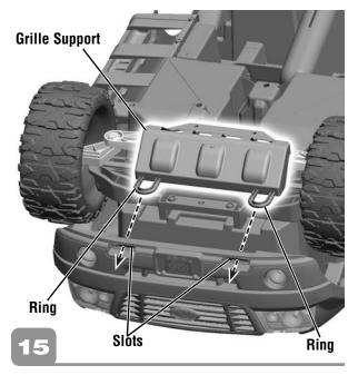
• Fit the rings on grille support through the slots in the grille. Push to **"snap"** the rings in place.
