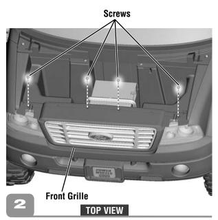
• Insert four screws into the top of the front grille and tighten.
