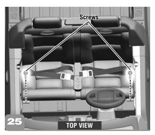
• Insert two screws into the tabs on the front edge of the seat and tighten.
