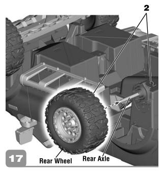
• Slide a rear wheel onto the rear axle.
