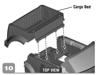
• Fit the tabs on the cargo bed into the slots in the back of the vehicle, as shown.
