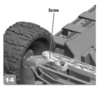
• Insert a screw through the large opening in the steering column cap and the hole in the steering column. Tighten the screw.
