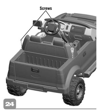
• Insert two screws through the back of the seat and into the vehicle. Tighten the screws.
