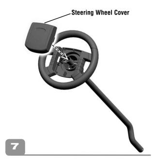
• "Snap" the steering wheel cover onto the steering wheel. *Hint:* If the steering wheel cover does not "snap" onto the steering wheel, you have not properly assembled the steering column to the steering wheel. Remove the pin and the steering column from the steering wheel and refer back to Assembly steps 5 and 6.
