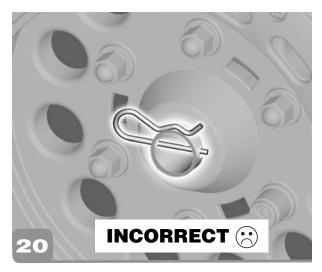
• If the clip is upside down or not through both holes in the axle, you have not assembled it properly. Please remove the clip and go back to step 18.
