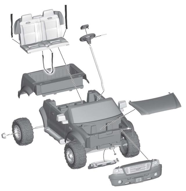
Note: Some parts shown are assembled to both sides of the vehicle. Fasteners not shown.
