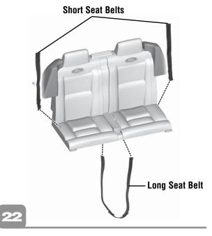
• Insert the "T" fastener end of a short seat belt strap down through the slot near the outer edge of the seat. Make sure the fastener side of the seat belt faces inward.
