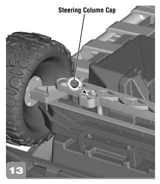
• Fit the steering column cap onto the end of the steering column.
