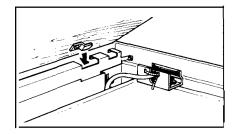
To remove the protective cover, use a scissor to cut the bag from the under side. Then reinstall the top taking care to engage the rear brackets as shown.
