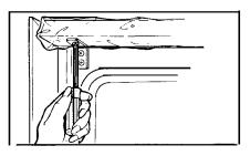
Remove the two mounting screws as shown and pull the top toward you to remove it from the dishwasher.
