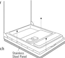
Door springs must be installed in the correct position.
