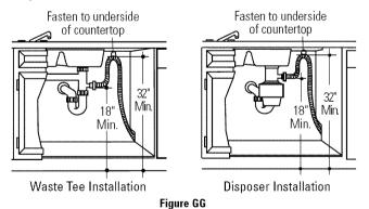
IMPORTANT — When connecting drain line to disposer, check to be sure that drain plug has been removed. DISHWASHER WILL NOT DRAIN IF PLUG IS LEFT IN PLACE.
