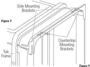
**IMPORTANT** — Drive screws straight and flush. Protruding screw heads will scratch the top or sides of the control panel and can interfere with door closing.
