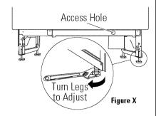
If adjustment to the right rear leveling leg is required, gain access by loosening junction box bracket screw (through the access hole) and rotate bracket clockwise.
