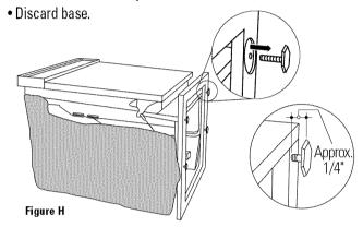
• Screw leveling legs back into the dishwasher frame, approximately 1/4" from frame as shown.
