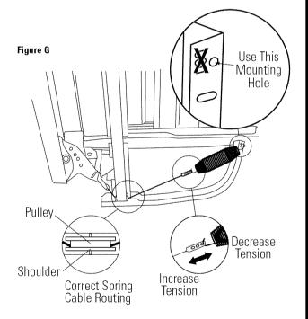
**TIP:** If door does not open easily or falls too quickly, check the spring cable routing. Check that the cable is properly aligned on the pulley (as shown).
