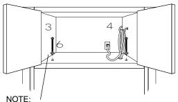
Screw length has been designed to accommodate 3/8" and above cabinet depth. If less, screw must be cut to required length.
