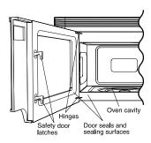
Check the oven for any damage, such as misaligned or bent door, damaged door
