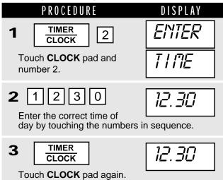
This is a 12 hour clock. If you attempt to enter an incorrect clock time, *ERROR* will appear in the display. Touch the **STOP/CLEAR** pad and re-enter the time.
