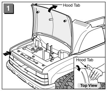
• Lift the hood to access the battery compartment. **Hint:** Place your hand on the vehicle body and "pop" the hood open by placing your hand under the hood tab
