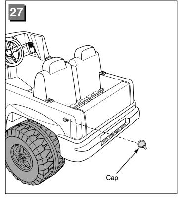
• Fit the cap into the hole in the side of the vehicle body.
