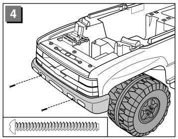
• Insert two #8-18 x 1<sup>3</sup>/<sub>4</sub>" screws into the holes in the front bumper and tighten.
