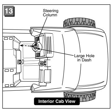
• Fit the end of the steering column out through the large hole in the dash.
