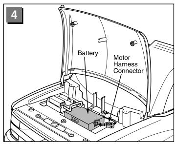
Plug the motor harness connector into the battery.
