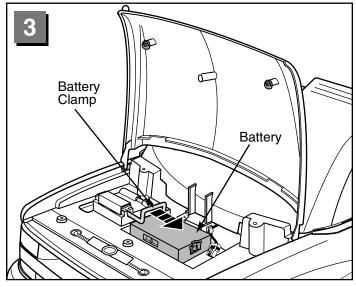
• Release the battery clamp. Make sure the battery clamp slides over the top of the battery. If the battery clamp does not slide over the top of the battery, reposition the battery in the battery compartment (see step 2).
