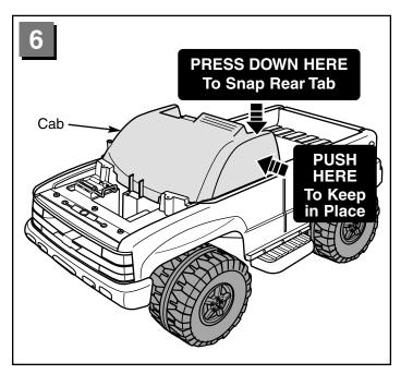
Press firmly above one of the rear tabs to snap it into the slot in the vehicle body.
