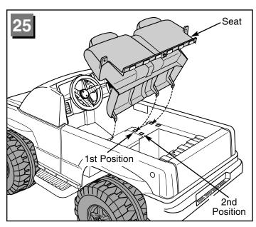
**Note:** The seat can be assembled in either of two positions for your child's comfort.
