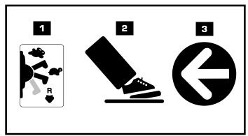
**IMPORTANT!** To avoid damaging the motors and gears, stop the vehicle before shifting from forward to reverse  $\blacksquare$ .
