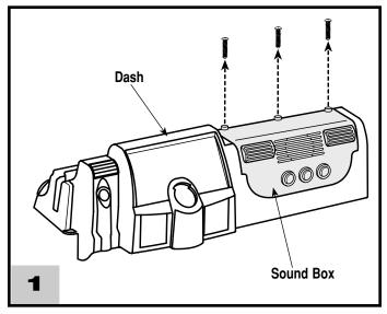
Loosen and remove the three screws in the top of the sound box.
