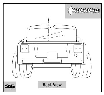
Insert a #8 x 1" screw into the rear edge of the seat. Tighten the screw.
