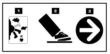
IMPORANT! To avoid damaging the motors and gears, stop the vehicle before shifting between low and high speed.
