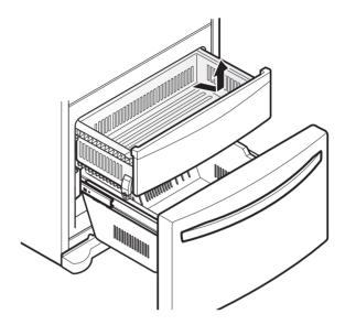
To reinstall, pull out and fully extend both rails. Insert the end of rib in the bracket at left and right. Making sure that the guides at the front are lined up properly, gently push down on both sides.
