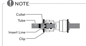
1) Gently press the Collet and insert the tube until only one line shows on the tube.
