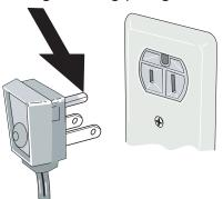
Power supply cord with 3-prong grounding plug
