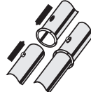
Positive Locking Wands Insert wand ends together until metal push button locks.
