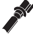
All Friction Fit Wands Insert wand ends together and twist to form a tight fit.
