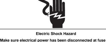
box or circuit breaker box. The dishwasher must be connected to a grounded metal, permanent wiring system. The equipment-grounding conductor must be run with the circuit conductors and connected to the appliance's equipment grounding terminal
