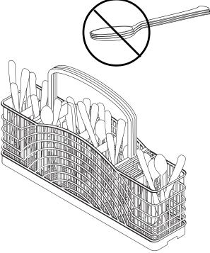
For safety, load sharp knives and forks with handles up.
