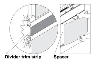
4. Check to see if spacer has remained in the channel of the divider trim strip. If it has not, replace securely in channel. It may be helpful to gently push in on divider trim strip while reinserting the spacer.
