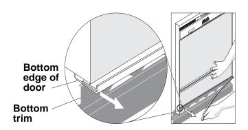
With one hand on the upper panel and one hand on the lower panel, gently slide the panel assembly down until the entire assembly rests on the floor. **Note:** Slide color panel(s) down about 1/2" on units without a divider trim strip.
