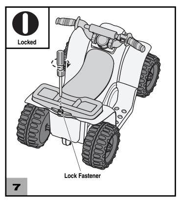
Using a slotted screwdriver, turn the lock fastener 1/4 turn to the locked position .
