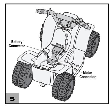
• Plug the battery connector into the motor connector.
