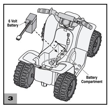
• Fit the Power Wheels® 6 volt (4.0 Amp/Hr) battery inside the battery compartment with the wires facing towards the rear of the vehicle.
