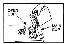
See "Detergent Usage Guide" below. (Be sure the Cycle Indicator Dial is at OFF position before adding detergent. Otherwise, the detergent cup will not close and latch properly.)
