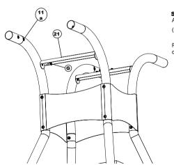
STEP 6 Attach seat (21) to back left leg (11a) using screws (G).
