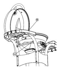
STEP 14 Attach left side shelf (6) to both side shelf legs (11) using screws (G).
