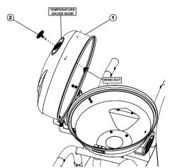
**STEP 12** *Note: Wing nut is packaged with temperature gauge.*
