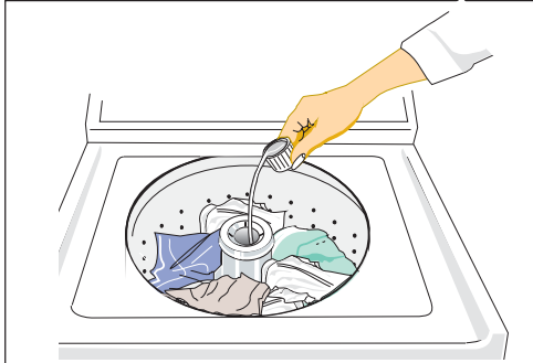
Built-In Fabric Softener Dispenser (some models)
