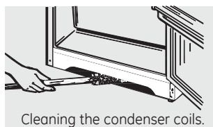
Cleaning the condenser coils.
