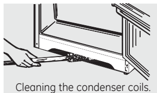
Cleaning the condenser coils.
