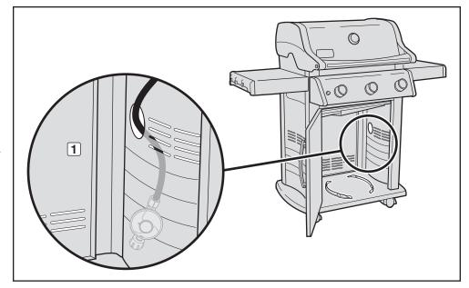
Maximum LPG cylinder capacity OUTSIDE cabinet is 13 kg.
