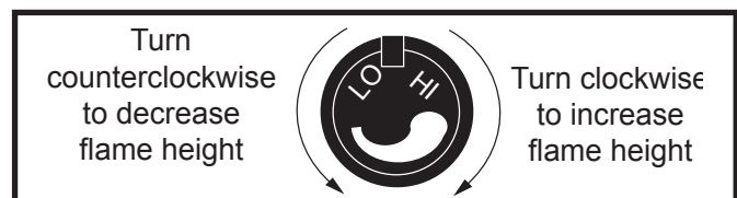
Fig. 42 Flame adjustment knob for Honeywell valve.
