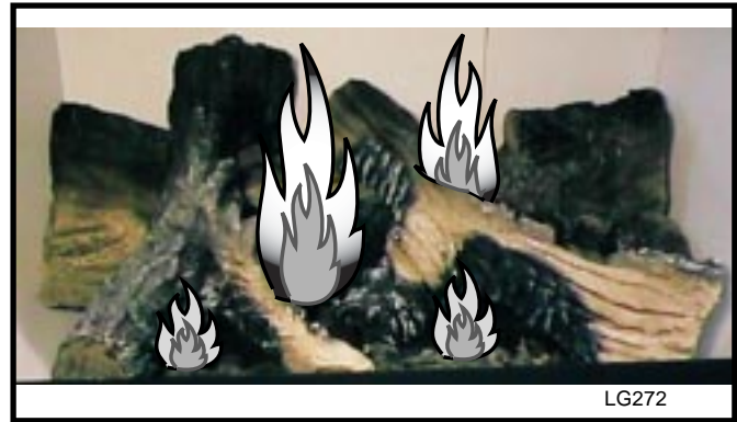
Fig. 46 Correct burner flame appearance for 36BDVR.
