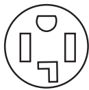
4-wire receptacle (14-30R)
