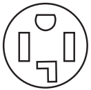
4-wire receptacle (14-30R)
