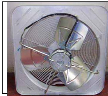
Fan and motor assembly Fig4-3
