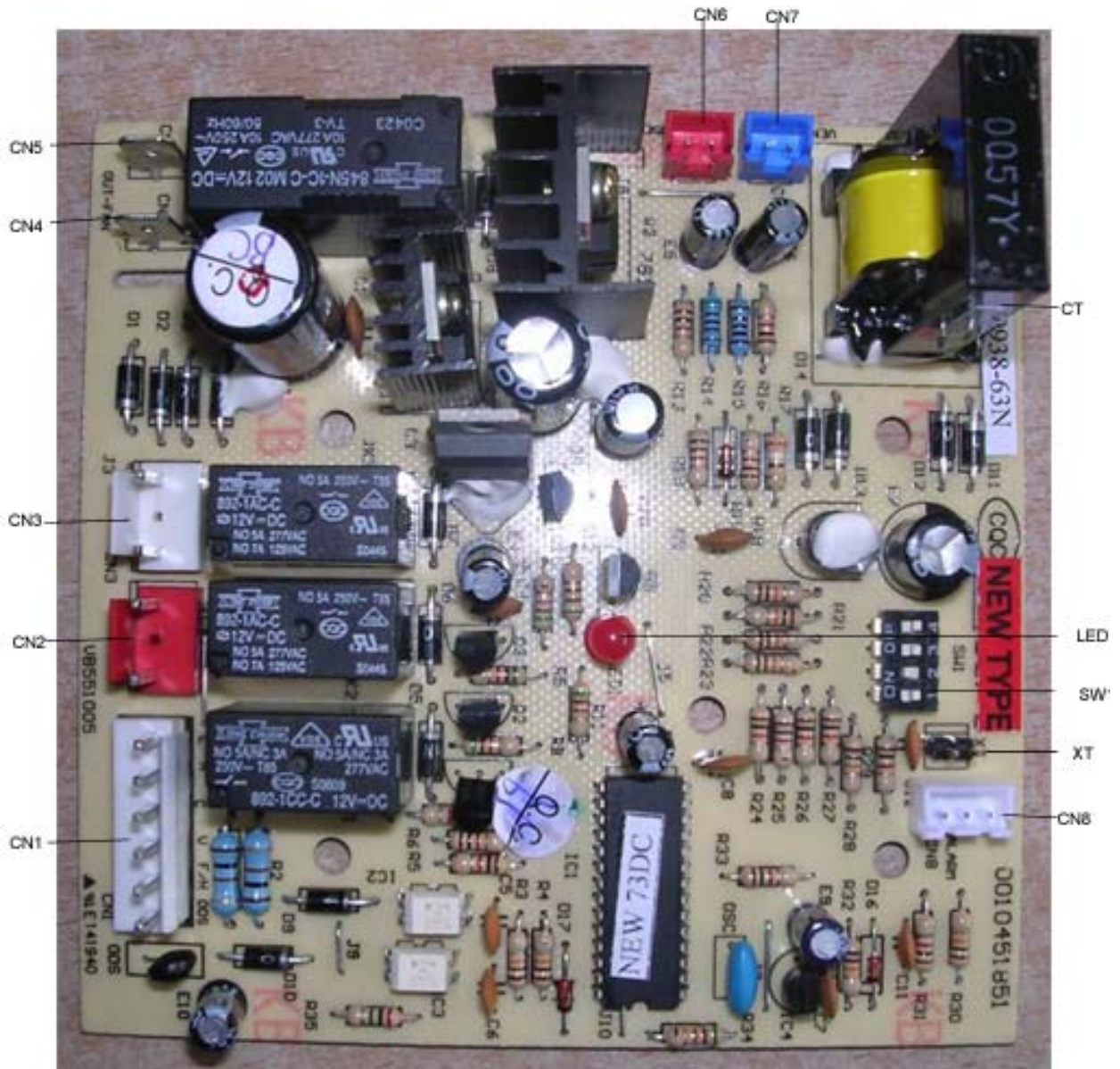
Heat pump control board
