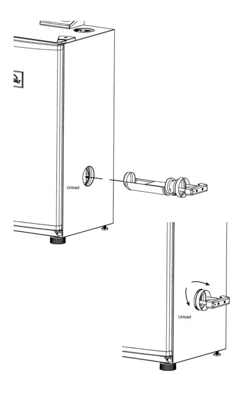
Before starting unit, place 1 cup of wood chips in chip loader.
