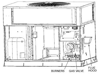
Fig. 2 — Gas Heating/Electric Cooling Unit
