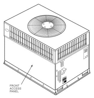
Fig. 1 — Gas Heating/Electric Cooling Unit (Unit 48GS Shown)
