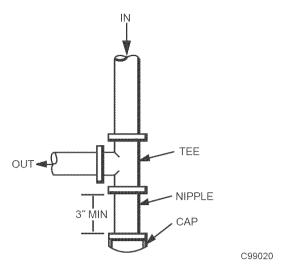
Fig. 9—Sediment Trap
