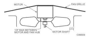
Fig. 12—Fan Blade Clearance
