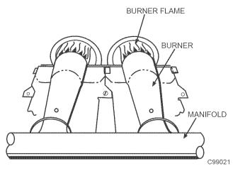
Fig. 14-Monoport Burner
