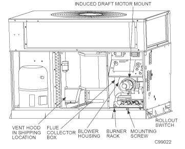
Fig. 31—Blower Housing and Flue Collector Box
