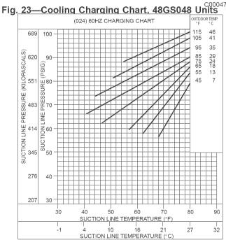
Fig. 25—Cooling Charging Chart, 48GX024 Units
