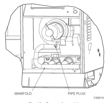
Fig. 13—Burner Assembly
