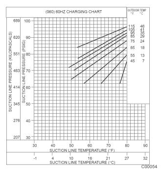
Fig. 30—Cooling Charging Chart, 48GX060 Units
