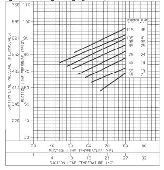
Fig. 21—Cooling Charging Chart, 48GS036 Units
