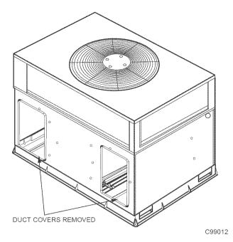
Fig. 10B-Vertical Duct Cover Removed
