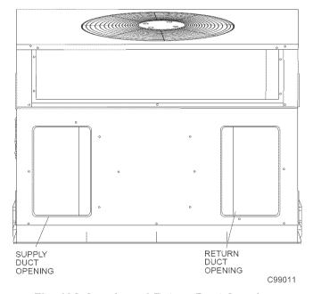
Fig. 10A Supply and Return Duct Opening
