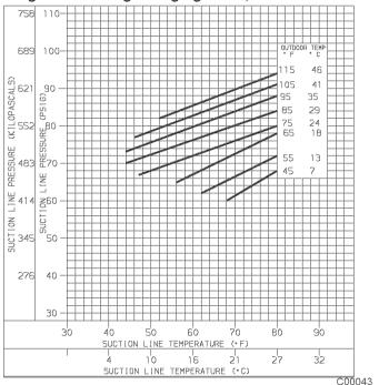
Fig. 20—Cooling Charging Chart, 48GS030 Units
