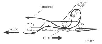
Fig. 7A—Threading Bolt for Rigging
