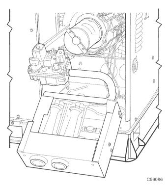
Fig. 34-Burner Rack Removed
