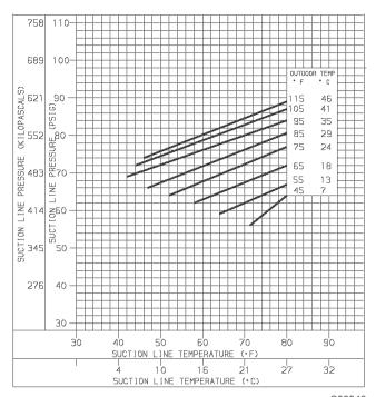
Fig. 19—Cooling Charging Chart, 48GS024 Units
