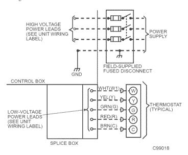
Fig. 11—High- and Control-Voltage Connections
