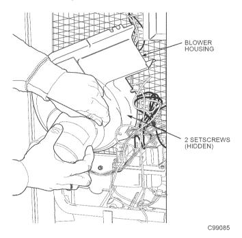
Fig. 33—Removal of Motor and Blower Wheel
