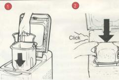
Special Note: If the baking pan is not installed in the proper orientation or firmly clicked into place the kneading blade will fail to operate!
