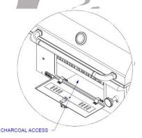
Charcoal grate assembly. Rotate the height adjustment knob to adjust the charcoal bed for multi-level heat control (see illustration to the right).
