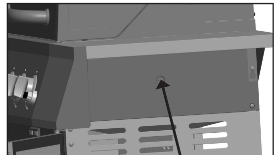
Hole for viewing the flame
