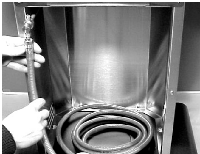
Figure 16 Natural Gas Hose Connection
