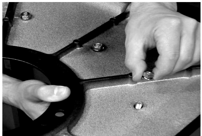
Figure 3 Attaching Pedestal to Base
