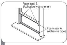
Cut the adhesive foam seal A and B strips to the proper lengths, and attach them to the window sash and frame as shown.
