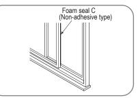
Cut the non-adhesive foam seal C strip to match the window height. Insert the foam seal between the glass and the window frame to prevent air and insects from getting into the room.
