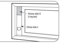
Insert the window slider assembly into the window opening.
