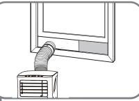
Insert the window slider adaptor into the hole of the window slider.
