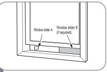
Insert the window slider assembly into the window opening.
