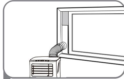
5 Insert the window slider adaptor into the hole of the window slider.
