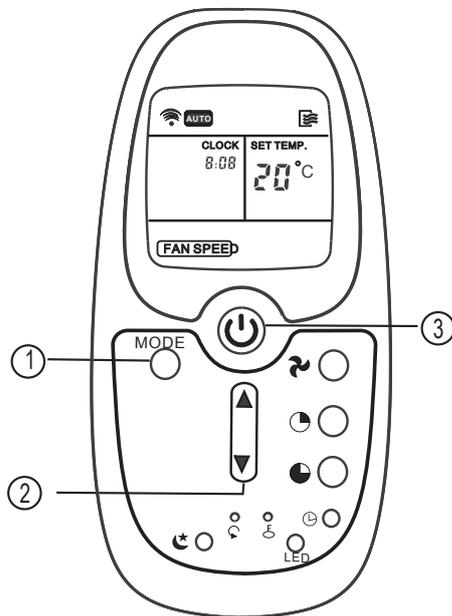
When you set the air conditioner in AUTO mode, it will automatically select cooling, or fan only operation depending on what temperature you have selected and the room temperature.
