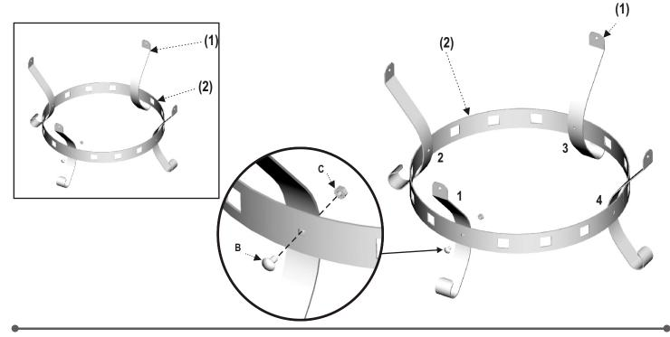
Making sure the legs (1) are on the inside of ring, attach legs to upper ring (3) as shown using 4X B from the outside and 4X C on the inside. Tighten nuts after all four legs are attached.
