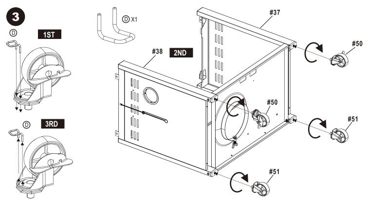
After all 4 casters are secure remove the Caster Pin (D) and save for future maintenance.
