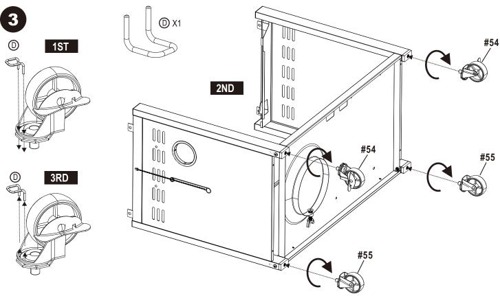
After all 4 casters are secure remove the Caster Pin (D) and save for future maintenance.
