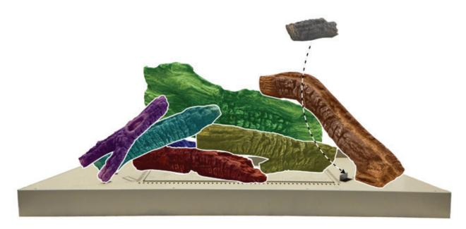
STEP 10. The log assembly is complete. Place glowing embers over the round ports on the burner as shown in Figure 3. Place ember sticks and coals on burner cover. Do not place ember sticks or coals over any burner ports. See Figure 4. Replace glass door and barrier screen as mentioned in fireplace manual.
