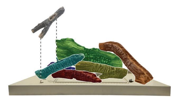
STEP 9. Place (Log Index Letter H) onto pin 8 under log F. See image below.
