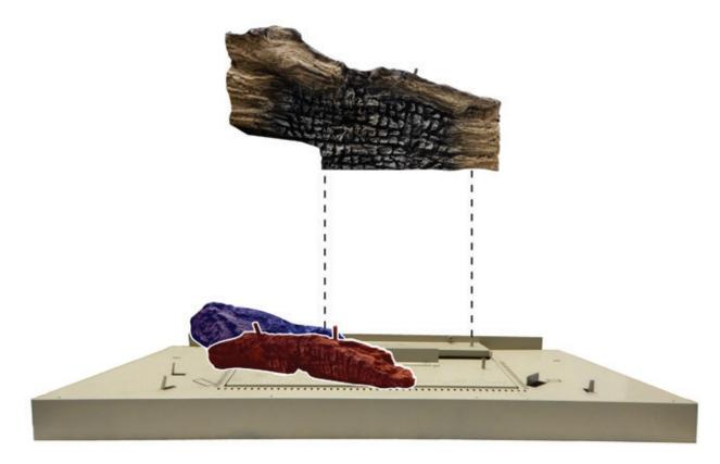
STEP 5. Place (Log Index Letter D) onto pin 3 and right pin on log B. See image below.
