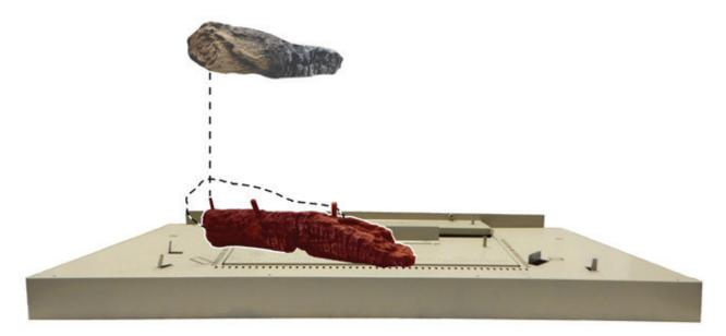
STEP 4. Place (Log Index Letter A) onto Pins 4 and 5 on the rear log support. See image below.
