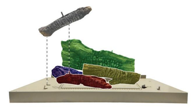
STEP 7. Place (Log Index Letter G) onto pin 9 on the burner and the pin on log A. See image below.
